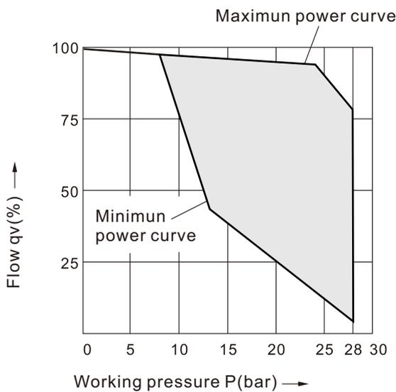
When ordering please state the power characteristics to be set at the factory in plain text,e.g.20KW at 1500rpm.
