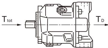
The split in torque between pump 1 and 2 is optional.
